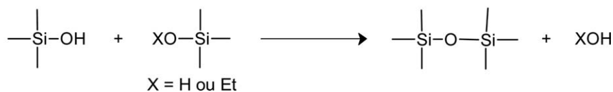
Scheme 1. Sol-gel reactions of tetraethoxysilane.
